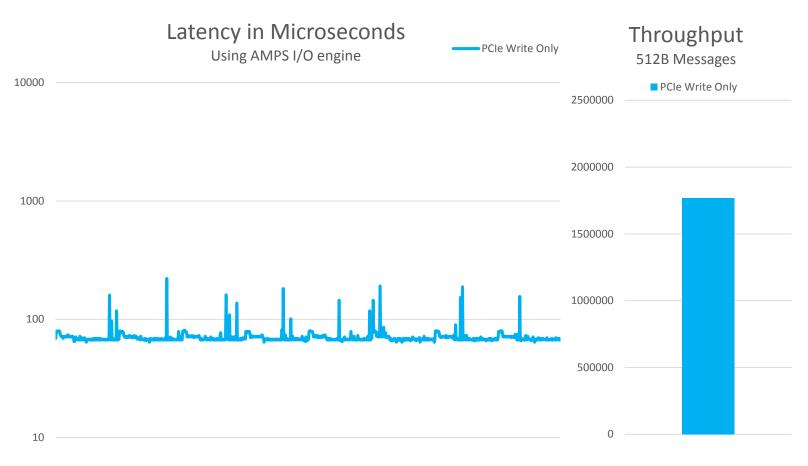
The overall throughput numbers are much better, and the latency is lower compared to the spinning disk: this is clearly a better solution for high-performance applications. The spinning disk had a wide variation in latency times. PCIe is more consistent, although it still suffers from regular spikes in performance. With 100% writes, the PCIe solution can handle nearly 1.8 million messages a second, or three times the number of messages handled by the spinning disk.
