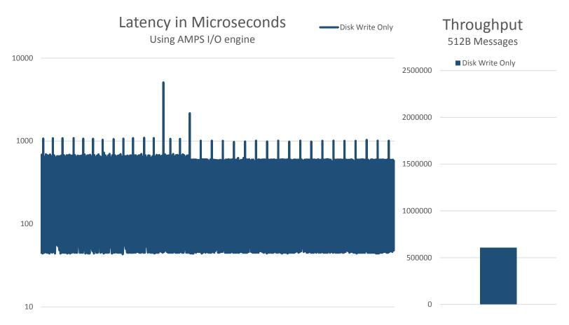
Notice that the latency chart uses a logarithmic scale: this is necessary because of the wide variance in numbers, and the fact that the numbers range from roughly 56µs to over 5ms. We use the same scale throughout this paper, to make it easy to compare the charts. Likewise, for the throughput chart, we use a consistent scale. The spinning disk can handle over 600,000 512B messages per second.
