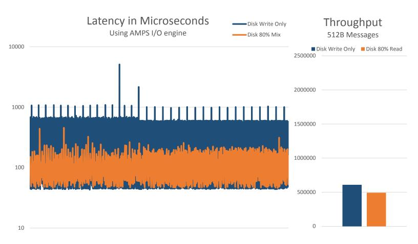
The latency drops somewhat when we add a heavy load of reads to the mix. However, this also reduces throughput to just under 500,000 messages per second. There's still a large variation in latency, though somewhat less than the write-only case.
