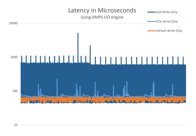
As you can see, latency is dramatically different for exFlash DIMMs overall. The latency is lower and more consistent than any other solution in the write only case.
