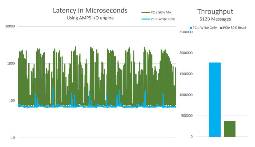
As with the spinning disk, though, when we introduce reads, both latency and throughput suffer. We ran the test again, changing the mix of operations from 100% write to 80% read and 20% write.
