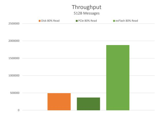
Both spinning disk and PCIe flash storage suffer a dramatic drop in throughput at the 80% read mix. eXFlash DIMMs, on the other hand, have only a slight drop in throughput.
